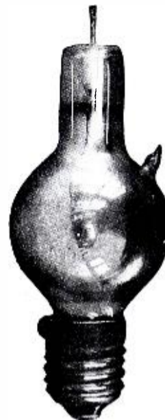
A typical rectifier tube of the Tungar type. The screw-base allows it to be inserted in a standard lamp socket from which current is obtained for the filament. Connection is made to the graphite disc by means of a Fahnestock connector which clips on to the wire post projecting from the other end of the tube.
