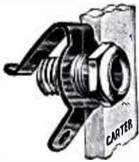
A tip jack which may be used for connecting loud speaker into the circuit.
