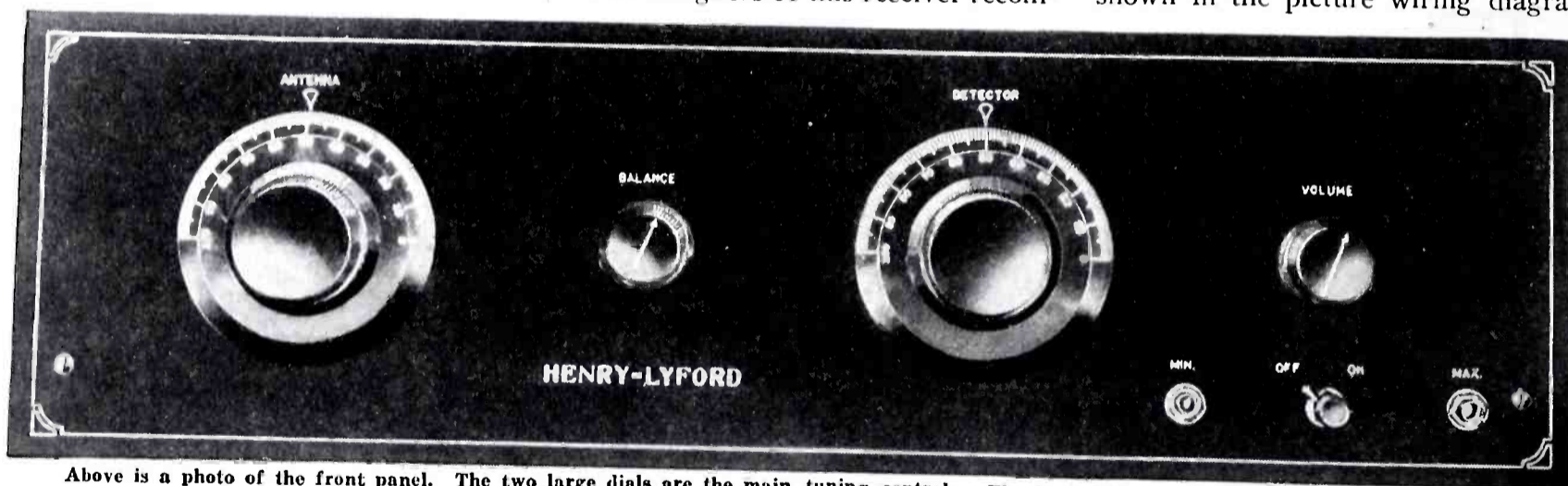
Above is a photo of the front panel. The two large dials are the main tuning controls. The knob between them is the balancing condenser and the one at the extreme right is the volume control.
